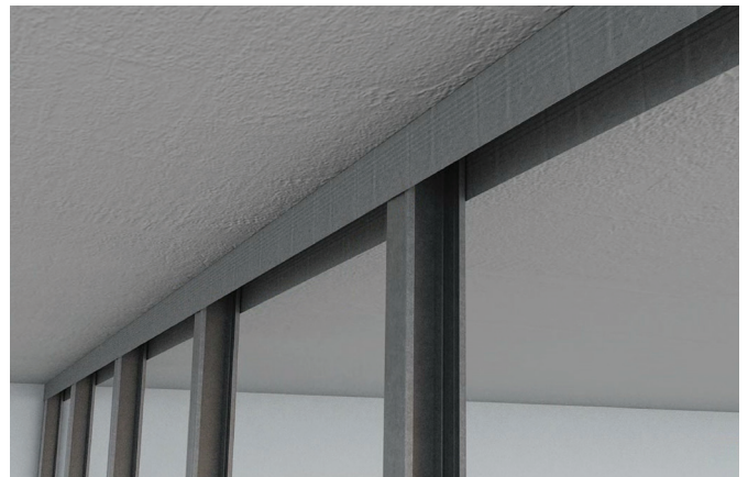
Step 4: Install intermediate C studs, spaced at maximum of 610mm using 12mm thick USG Boral Standard board. The studs open face should face a single direction.
